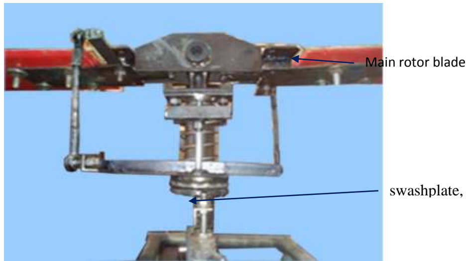
Figure 3: Construction and installation of the swashplate.
