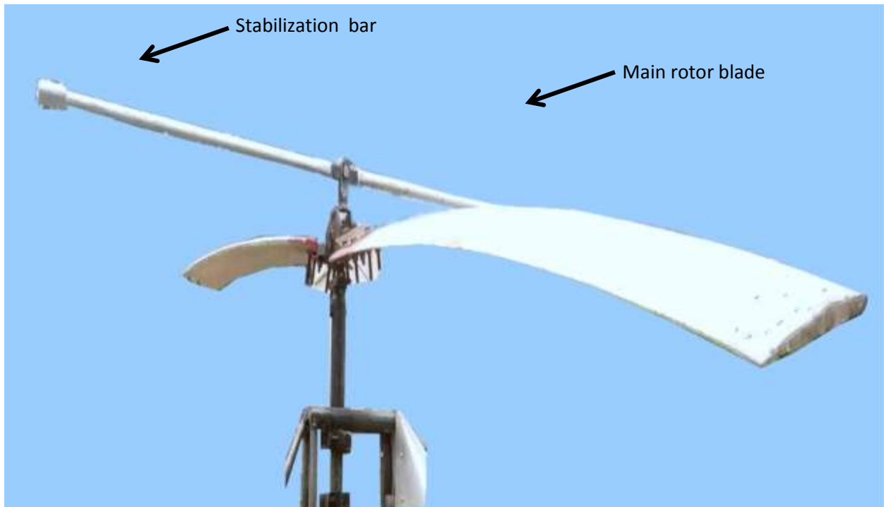
Figure 2: Realized and mounted main rotor blades.
